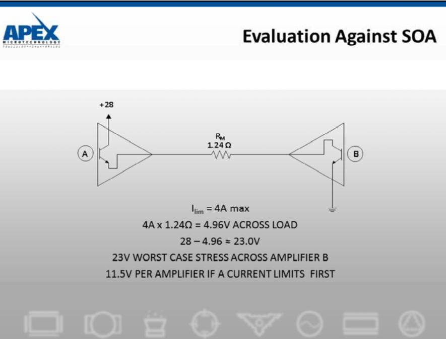
The above model provides us with a tool for analysis to examine worst case SOA stresses. This represents the condition for motor start-up or stall (not as demanding as instant motor reversal which is easily avoidable).
