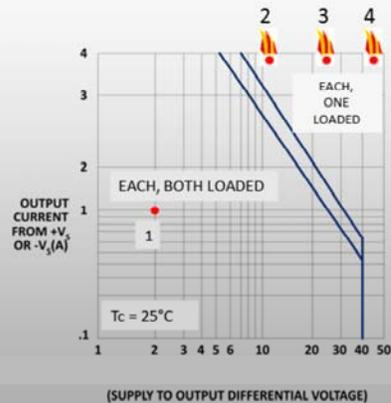
Plotted on the PA74 SOA graph are the four possible operating conditions for the PA74 when used with the Electro-Craft E540.
