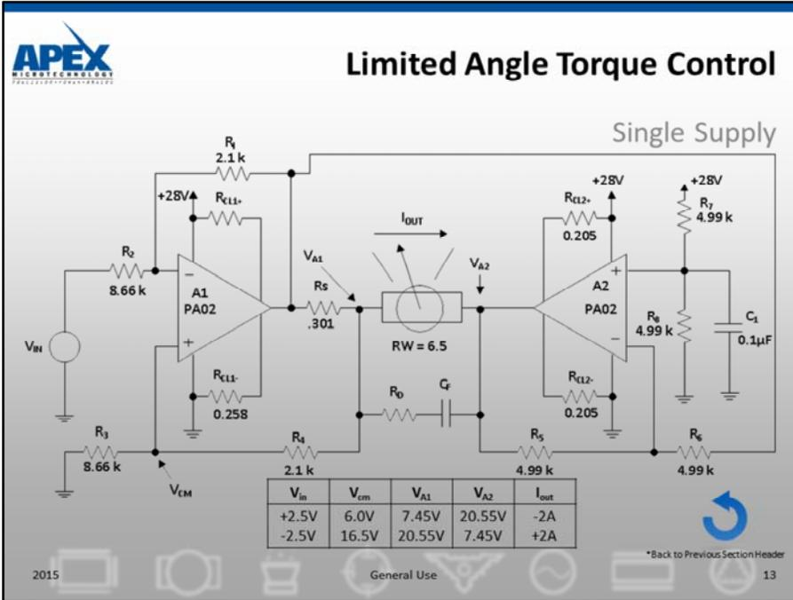
This real world application shows implementation of the generic case of V to I single supply. It combines bridge mode operation with the improved Howland current pump. The limited angle torquer will see bipolar current changes for bipolar input voltages.
