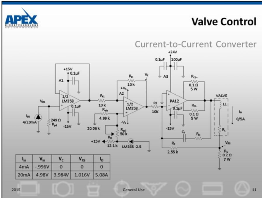
This circuit provides a Current-to-Current converter function through translation of a 4-20mA current transmitter to 0-5A output for linear control of a valve.
