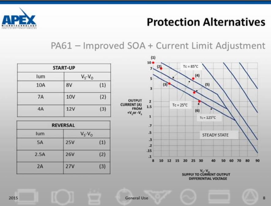
Often the only solution to the conflicting requirement of protection along with reasonable motor acceleration is simply an amplifier with a larger SOA. Not only does the PA61 provide a better SOA fit but the programmable current limit provides additional flexibility in meeting SOA requirements.
