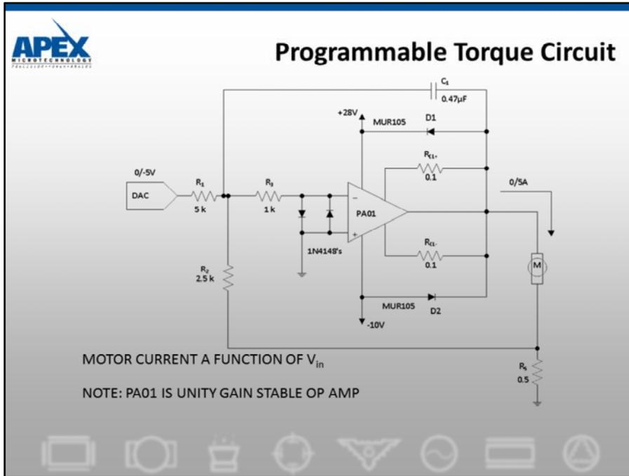
This schematic uses several tricks that we've learned. First of all, notice that the PA01 is operating from non-symmetrical supplies. The  $-10$  volt supply is merely to provide input common mode bias. The  $28$  volt supply is used to supply the load current.
