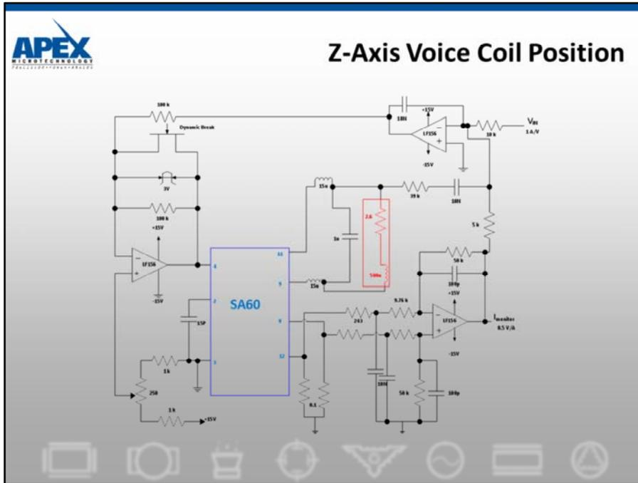
Slower versions of this machine used a PA12 linear op amp for Z-axis control. Even though currents were lower and motor impedance was higher, an exotic custom heat sink had to be designed to fit the small physical location of the amplifier. It was clear that this generation of the machine required higher efficiency in the drive circuit. The SA60 provides this and being programmed to switch at about 220KHz, it provides adequate bandwidth for the high speed servo loop.
