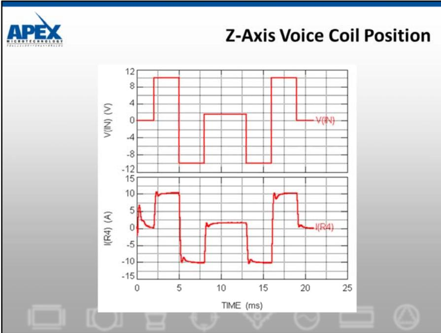
After power up settling, the first 3msec pulse accelerates the motor toward the work piece; the second 3msec pulse decelerates the motor; a constant pressure is held for 60msec (time was compressed in this plot); the last two pulses move the motor back to home position; and at t=150msec the cycle is repeated.
