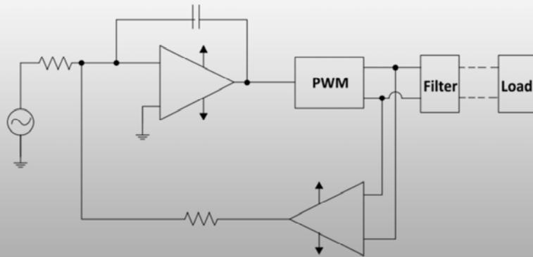
This simple voltage control circuit illustrates that in addition to improving accuracy over open loop operation, the integrator simplifies circuit design. Assume the input and feedback resistors are equal and that the gain of the differential feedback amplifier is  $1/10$ . This tells us right away that the circuit gain is 10.
