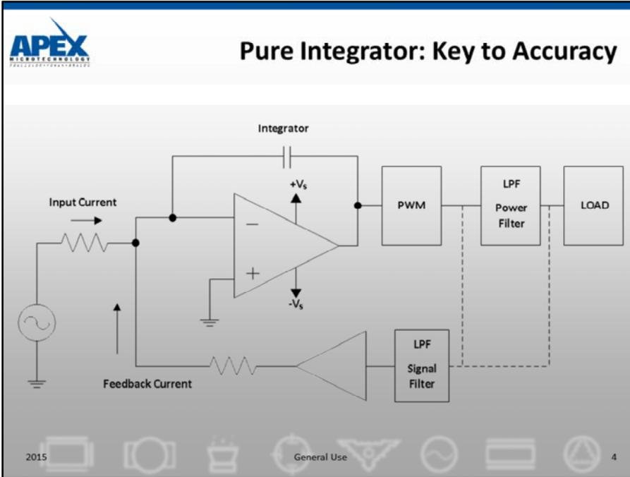
Here is very general look at closing a PWM amplifier locally. The PWM output is filtered and delivered to the load as a power analog signal (occasionally a load may do its own filtering). A feedback circuit usually contains a low pass filter and often an amplifier. It has multiple topology options to monitor voltage, current or process variables such as position or temperature. The feedback circuit provides a voltage representation of the job actually being done.
