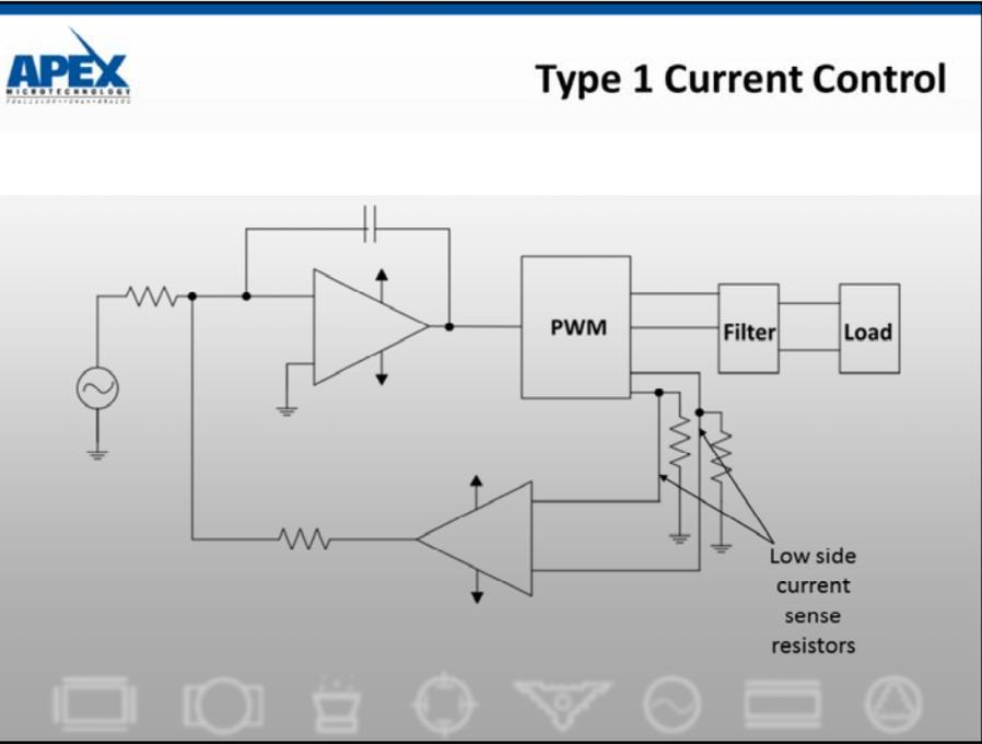
Remember the four switches configured as an H-bridge? Underneath the two lower switches, we insert low value sense resistors to monitor current. As the load current changes polarity, the current path switches resistors. With a differential amplifier looking at both resistors, it will output a bipolar voltage corresponding to the bipolar current in the load.
