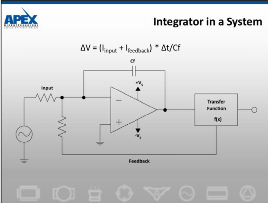
With a little modification, we can transform this switching circuit into a very useful linear tool. What is required is a form of feedback to maintain operation in the transition area, or the linear area. This figure shows a generalized form of this where  $f(X)$  is non-inverting. This function is often non-linear, but seldom contains step functions.
