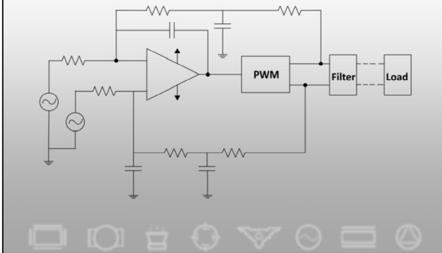
By substituting a second PWM output for the voltage reference of the previous circuit, and adding a low pass power filter, we have simple control of a high power drive with a minimum component count.
