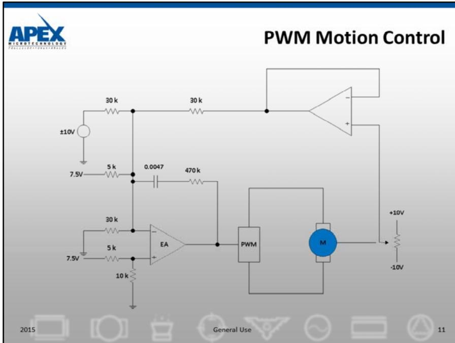
While one of the simplest forms of position sensing is shown here, options such as optical encoders, LVDT sensors, tachometers and variable capacitance transducers are all viable ways to sense speed or position. In a wider sense, this basic circuit can be adapted to control a wide variety of process variables such as temperature, flow rate, pressure, light intensity.....
