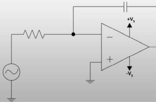
No, this slide is not a mistake, its just a way to examine the basic operation of the op amp integrator.
