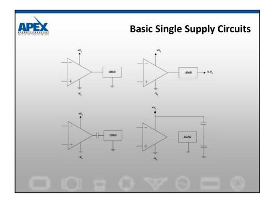
Circuit A is only suitable for unipolar and non-zero inclusive drives. These type applications might include Programmable Power Supply (PPS), heater controls and unidirectional speed controls.
