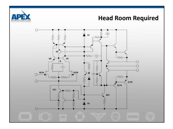
Notice that as the input pins approach the negative rail, the voltage across Q15 decreases. Minimum operating voltages for Q12 and Q15 along with the zener voltage place a limit on how close common mode voltage can get to the negative rail.
