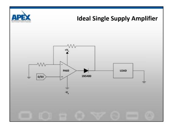
The PA60 series amplifiers feature a common mode voltage range from 0.3V below the negative supply rail (ground in this case) to with in 2V of the positive rail. These amplifiers also swing to about 0.5V of the rail with very light loads making the diode level shifter above quite practical as long as the load is resistive. With the diode inside the feedback loop it contributes essentially no errors at the load.
