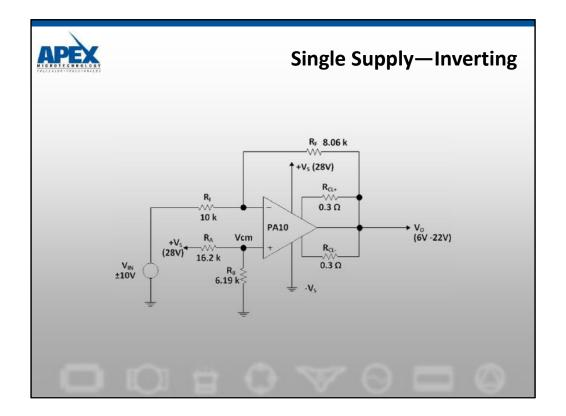
GIVEN: Vs= 28V  $Vin = \pm 10V$   $\{1+(Rf/Ri)\}$  Vo = 6V 22VFIND: Scaling resistor values \*RB)/(RA+RB)}  $\{1+0.8\}$  **STEP 3:** Offset: Set Vin =0, Vo=14V Vo= -Vin(Rf/Ri) + {(Vs\*Rb)/RA+RB)}
