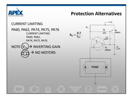
This handy circuit can be used with the PA60 series amplifiers in a single supply application to provide external current limit with minimum components.
