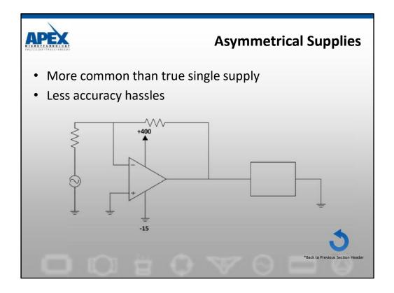
There's something very appealing about a circuit with only two gain setting resistors. Many times there is already a low voltage supply in the system just waiting to be used. This supply need only provide quiescent current of the op amp unless the op amp swings negative or in the case of reactive loads where current and voltage are not in phase.
