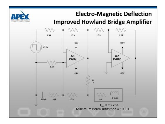
A1 is a Howland Current Pump, A2 provides a gain of -1 to drive the opposite terminal of the coil. A first glance, it might appear the choice of  $2\Omega$  for the sense resistor is quite large because the peak voltage drop across it is 7.5V, or half the supply voltage. Voltage across the inductor required to move the beam is given by: VL = L \*  $\Delta I / \Delta t VL = 300\mu H * 7.5A / 100\mu s = 22.5V$
