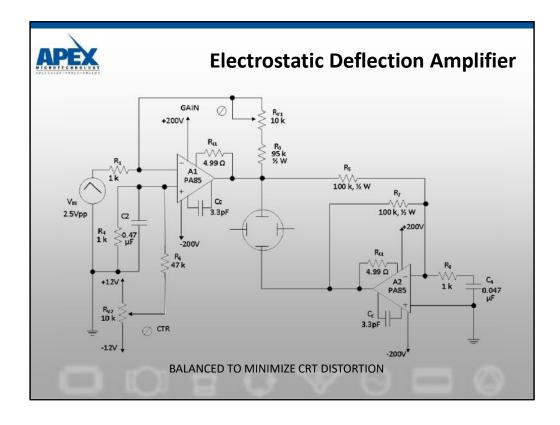
The PA85 was chosen for this application for its high voltage and high speed characteristics. Full bridge drive is utilized to provide a balanced drive to the CRT plate. Bridge drive is useful to reduce geometric distortion in electrostatic deflection applications.
