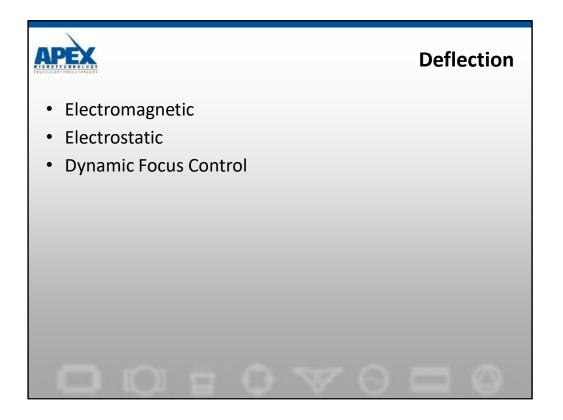
High speed power op amps are ideal candidates for all types of deflection uses. High current, high speed models are ideal for electromagnetic deflection. Models with rapid slew rates and extended supply ranges allow rapid dl/dt of the yoke being driven. High voltage models are especially useful for electrostatic deflection and/or focus.
