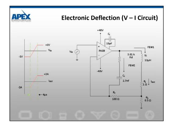
Amplifier Selection:Step 1: Voltage $V_{LL} = LL \frac{Dip - p}{dt}$  $V_{LL} = 13 \mu H \frac{4A}{4\mu s} = 13V$  $V_{S} = V_{LL} + V_{RL} + V_{RS} + V_{sat}$  $V_{SMIN} = 13V + 2V + 1V + 8V$ Where:  $V_{RL} = Ip RL$  $V_{SMIN} = 24V$  $V_{RS} = Ip Rs$  $V_{SMIN} = 24V$
