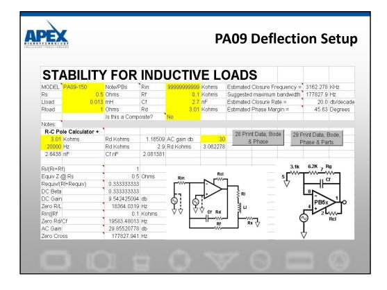
Set up the basic circuit in Power Design to see we have a 17 degree phase margin. Visualize the flat portion of feedback path #2 at about 30db. This is well below the intersection point and gives a nice round gain increase of 10x or 30 total. Estimate the line will cross the closed loop gain at about 200KHz.
