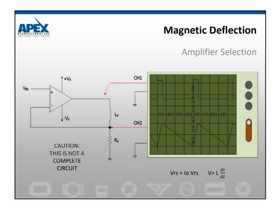
An amplifier selected for magnetic deflection must have an adequate slew rate and voltage rating to slew the current in the yoke fast enough.
