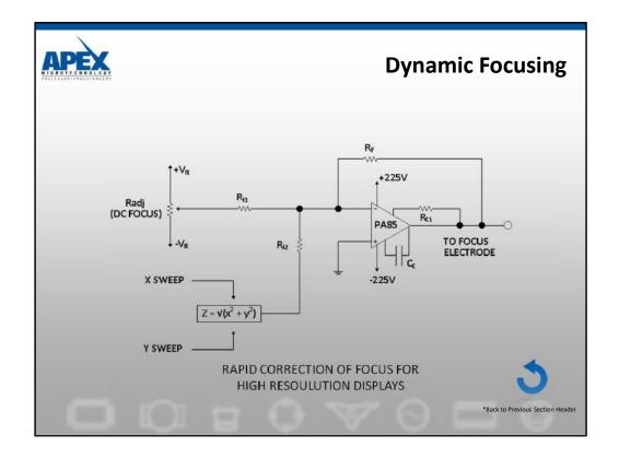
In a flat screen display system the distance from the source of the beam to the screen changes as it deflects on the screen, from left to right, and from top to bottom. As a result of this a dynamic focus is required to keep the beam in focus, no matter where it is located on the screen.
