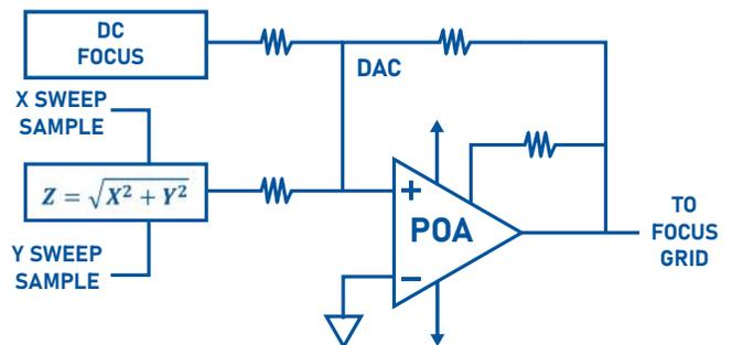
By offering multiple combinations of high speed and high voltage power amplifiers, Apex can drive the rapid correction of focus in high resolution displays. Dynamic focusing is the active correction of focusing voltage as a beam moves from the center to the edges of a CRT. Power operational amplifiers lend themselves well to this application with their ability to be connected as a summing amplifier with inputs from the nominal focus potential and the dynamic correction.
