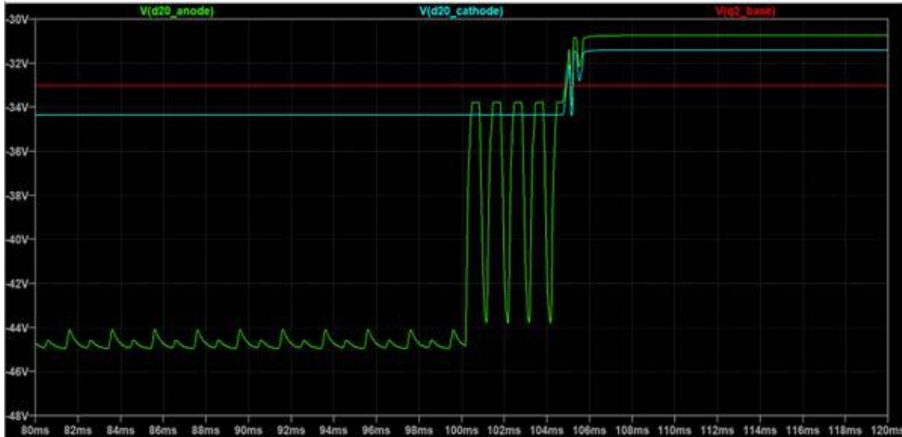
Figure 5: Voltages Across D20 During Normal Operation and Current Limit with \pm 45\text{V} Supplies
