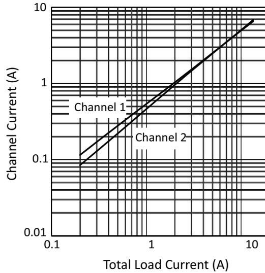
The uneven distribution of current on the low end of the scale is likely due to thermal equilibrium, which is discussed in later sections. This experiment demonstrates that the two top FETs on the same monolithic chip do NOT have identical properties, but they are closer-matched than two discrete FETs selected at random.
