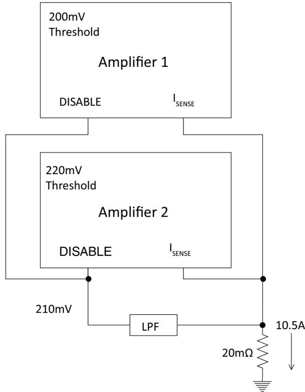
Instead, there must be a network that senses current and produces a signal that supersedes any variation in threshold voltages. This can be accomplished by adding a level-shifting comparator to the mix.
