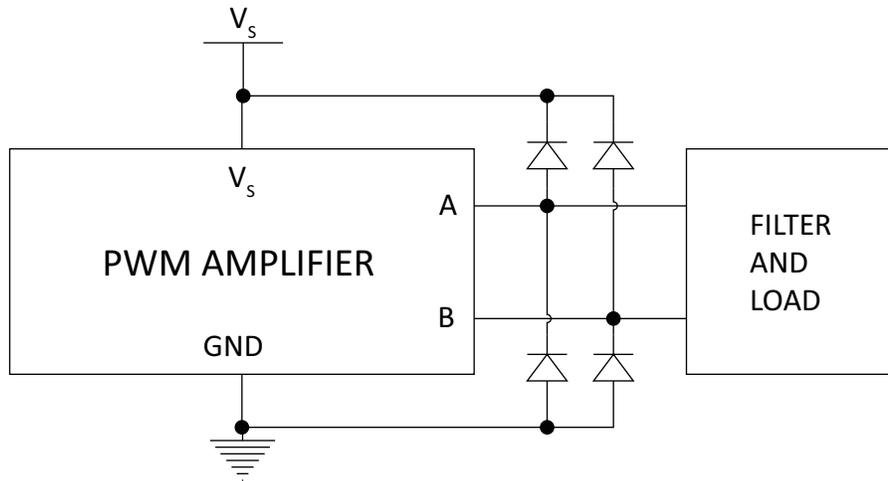
Recall that the purpose of these diodes is to “snub” inductive voltage spikes so they do not reverse-bias the MOSFETs and damage the parasitic body diode. Even if the load is purely resistive, the inductance in circuit traces and wires is enough to make some considerable voltage spikes when combined with the  $di/dt$  associated with Apex switching products.
