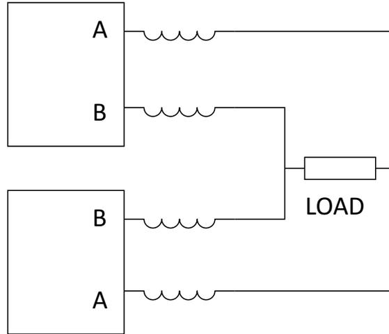
Not only do these inductors serve as a filter to demodulate the PWM signal, but they temporarily limit the current in the event of asynchronous turn-on/-off conditions. To determine the appropriate value of inductance, a first-order filter can be designed using Apex Power Design or the equation in AN30 section 5.2 “How Much Inductance?”. For these techniques, design the filter for twice the load resistance; the filter will be duplicated on each amplifier.
