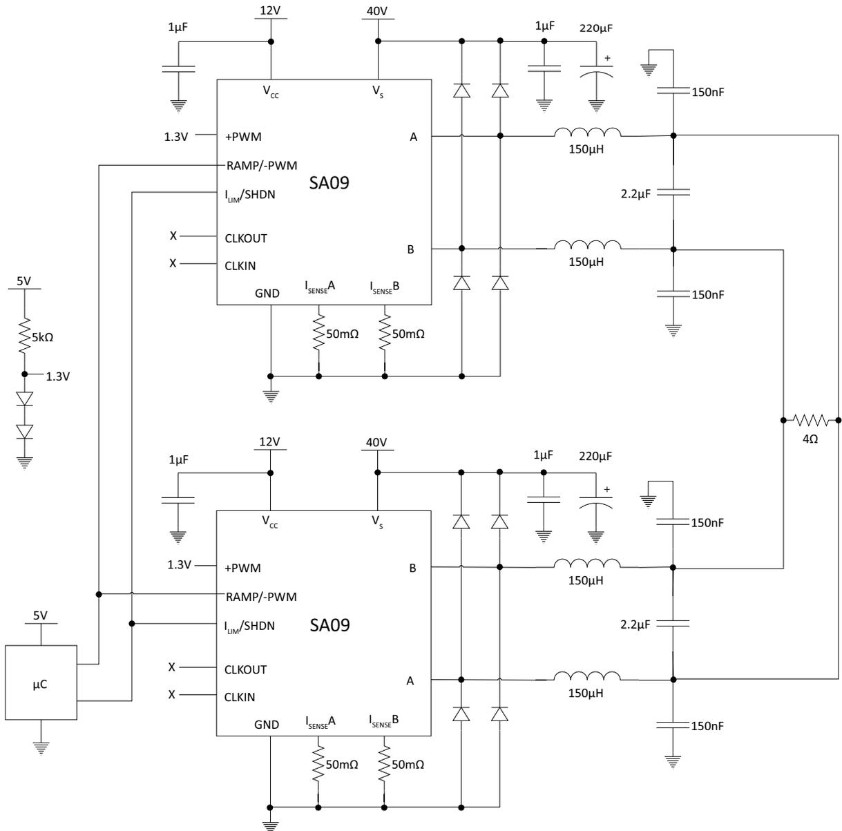
In this example, a 2<sup>nd</sup>-order filter was designed (for an 8  $\Omega$  load with 6 kHz cutoff frequency) using Apex Power Design. This yields inductors of 150  $\mu\text{H}$  and a capacitor of 2.2  $\mu\text{F}$ . The equation for minimum inductance (above) indicates that at least 2.3  $\mu\text{H}$  is required; this is satisfied by the 150  $\mu\text{H}$  from Power Design.
